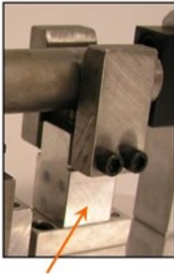
RB02 4 Holed altered to create gooseneck post using Rapid Plates™
